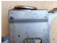
Top mounting plate distortion as a result of a single significant impact or multiple lower level impacts. Even if the rest of the castor is in good condition, it must be replaced.
