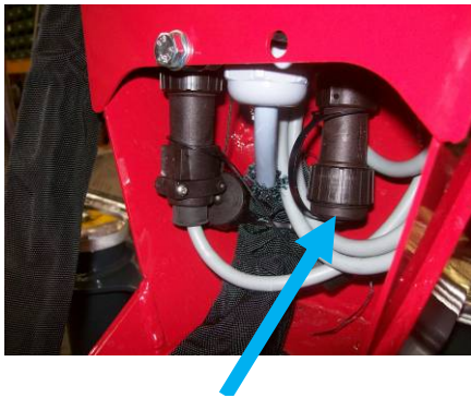
Remote control power cable
